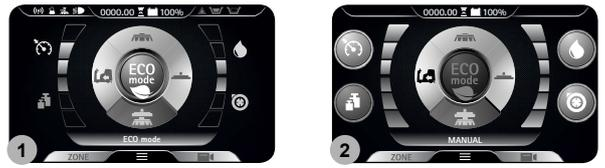
In the middle of the DS selector there is the ECO-MODE button (1), if in any eco-mode program you press the button (1) you pass from ECO mode to MANUAL mode, with manual management of the individual parameters.
