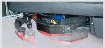
Retractable 10 cm offset disc deck enhances edge scrubbing and resists damage from accidental impact
