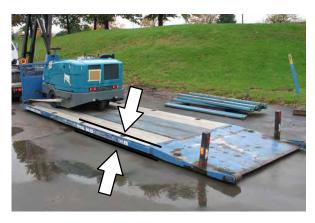
To winch the machine onto the truck or trailer, attach the winching chains to the holes in the right and left lower corners in front of the machine.
