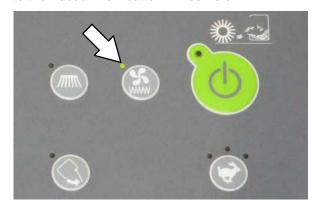
NOTE: Turn off the vacuum fan when sweeping over large wet areas or standing water. This prevents the dust filter from getting wet while sweeping.
