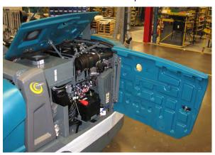
2. Loosen clamps securing the cover to the HEPA filter assembly and remove the cover from the HEPA filter assembly.
