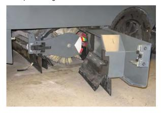
3. Unlatch and remove the brush idler plate.
