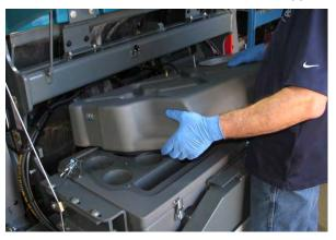
3. Disconnect the main wire harness from the filter shaker assembly jumper cable.
