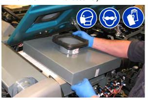
3. Remove the HEPA filter from the HEPA filter compartment.
