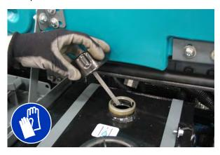
Machines (S/N 007685- ) have a fluid level gauge on the hydraulic tank. The hydraulic fluid level should be between the two lines on the hydraulic gauge.
