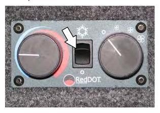
Use the *Temperature knob* to control the cab heater temperature. Use the *Fan knob* to control the air conditioner temperature.
