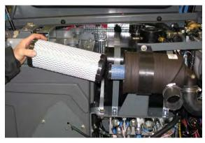
Replace the safety filter element after the primary has been changed three times. Do not remove the safety filter element from the housing unless it is restricting air flow.
