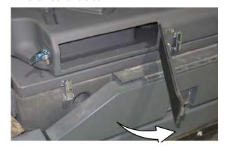
4. HEPA Machines: Use a HEPA certified vacuum to clean dust and debris from the interior of the upper cyclone chamber.
