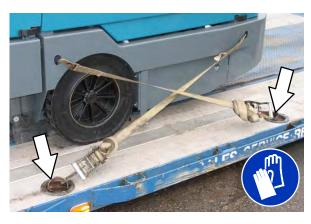
FOR SAFETY: When unloading machine off truck or trailer, use winch. Do not drive the machine off the truck or trailer unless the loading surface is horizontal AND 380 mm (15 in) or less from the ground.
