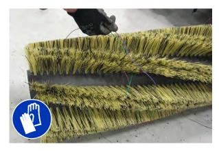
Rotate the brush end-for-end after every 50 hours of operation, for maximum brush life and best sweeping performance. Refer to REPLACING OR ROTATING THE MAIN BRUSH.
