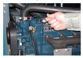
Fill the engine with oil until the oil is between the indicator marks on the dipstick. DO NOT fill past the top indicator mark. The engine oil capacity is 6 L (6.35 qt) with oil filter.
