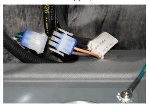
4. Disconnect the ground wire from the lower cyclone chamber.
