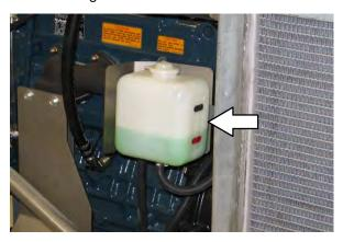
FOR SAFETY: When servicing machine, do not remove cap from radiator when engine is hot. Allow engine to cool.
