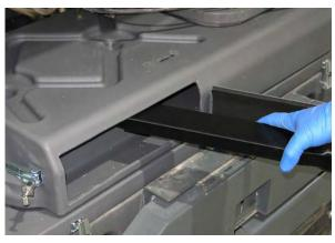
HEPA Machines: Use a HEPA certified vacuum to clean the slots located at the top of the dust filter compartment.
