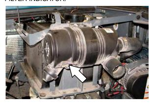
Remove the filter element. Carefully clean the end cap and the interior of the housing with a damp cloth. Clean the housing sealing surfaces.
