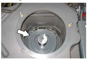
2. Open the rear cyclone cover access port to empty dust and debris from the cyclone cover.
