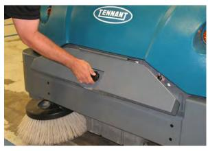
Pull the hopper access door handle to open the hopper access door. (SN 006501 – )
