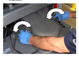
4. Disconnect the vacuum hose from the dust filter cover.
