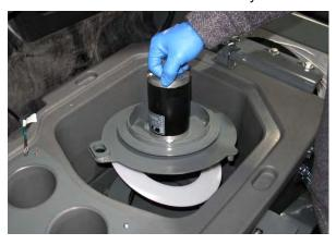
7. Loosen the three clamps securing the lower cyclone chamber to the hopper.
