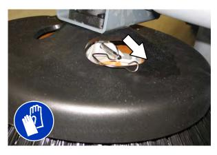
NOTE: Remove the drive hub and put it on the new brush if one is not installed.
