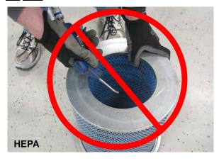
Inspect the dust filter seals for proper seal and damage. Dust build up on the seal surfaces means dust is getting past the dust filter, significantly reducing the HEPA filter life.
