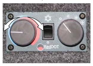
Use the *Fan knob* to control the fan speed. This knob affects the heater and air conditioner.
