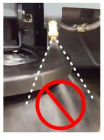
To adjust the spray pattern, use the water valve located under the water tank. Do not open the valve to the  $90^{\circ}$  maximum position. Optimal position is with the valve opened between  $10-15^{\circ}$
