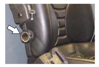
The weight adjustment knob controls the firmness of the operator seat. Use the gauge next to the weight adjustment knob to help determine seat firmness.
